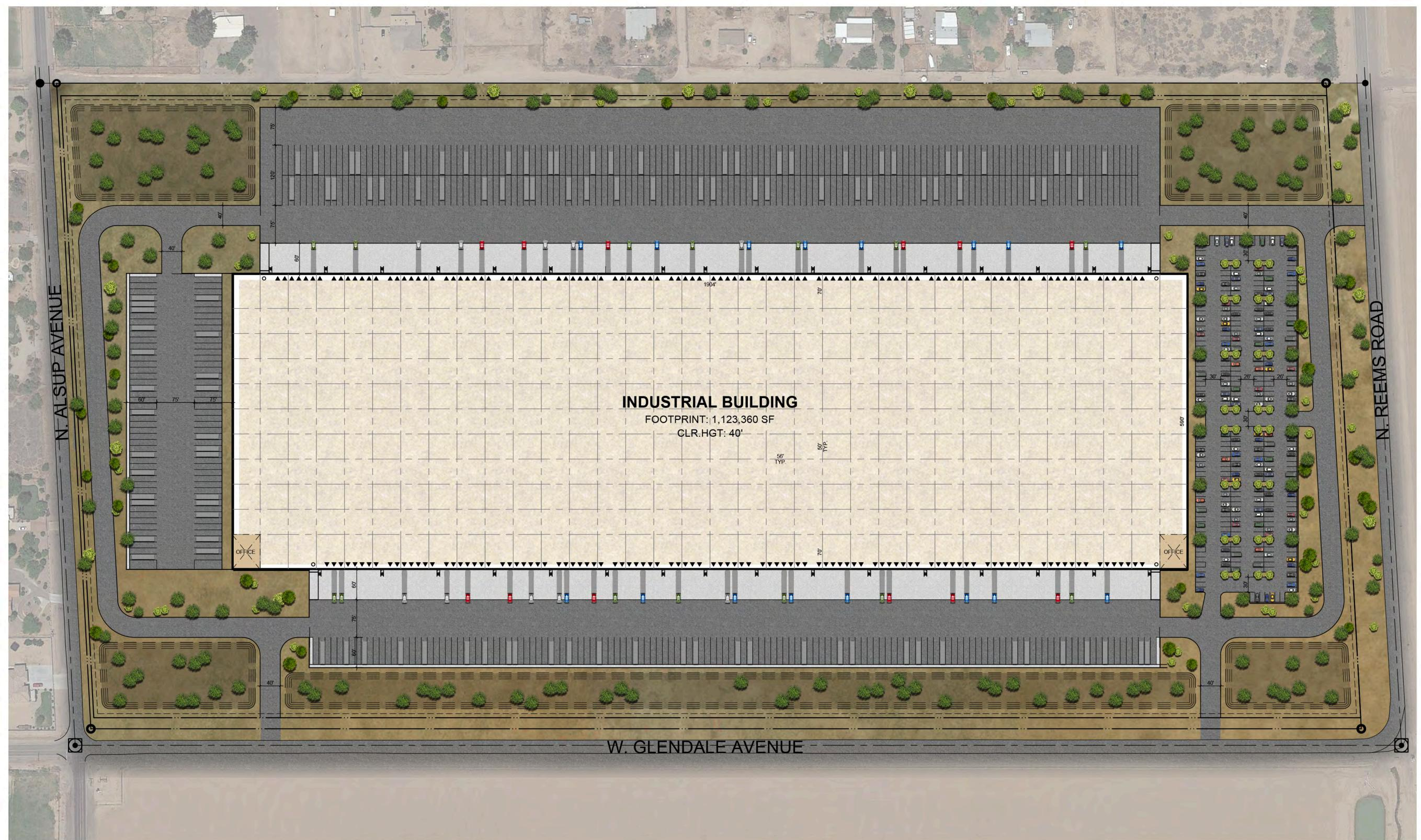
PROJECT DATA: SITE AREA: 74.64 AC GROSS: 3,251,318 SF **DETENTION:** SLOPE: EASEMENTS: OUT-PARCEL: NET: 65.76 AC 2,864,720 SF BUILDING FOOTPRINT: 1,123,360 SF 99,120 SF BUILDING AREA EXPANSION: COVERAGE: GROSS: 35% NET: PARKING PROVIDED: AUTO: 345 STALLS @0.31/1000 SF 8 STALLS REQ. ACCESSIBLE TRAILER: 518 STALLS TRUCK DOCKS: ▲ DOCK-HIGH DOORS 212 O GRADE-LEVEL DOORS
