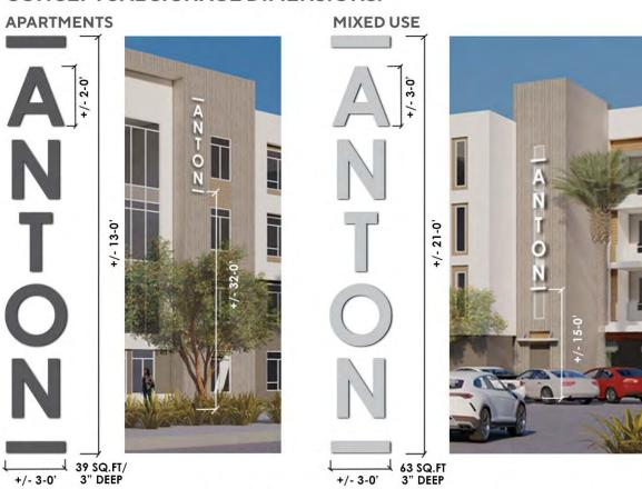
**Design:** Internally illuminated vertically stacked channel letters that are attached to the building facade. The channel letter color scheme will be complementary color(s) to the City of Glendale's approved exterior paint color for the project. Initial design is considering a dark or light tone for the letters. Both signs will be visible from 99th Ave. Signage is of aluminum construction.
