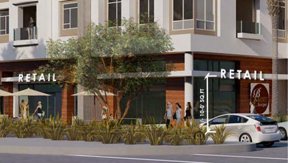
**Design:** Internally illuminated vertically stacked channel letters that are attached to the building facade. The channel letter color scheme will be complementary color(s) to the City of Glendale's approved exterior paint color for the project. Initial design is considering a dark or light tone for the letters. Both signs will be visible from 99th Ave. Signage is of aluminum construction.
