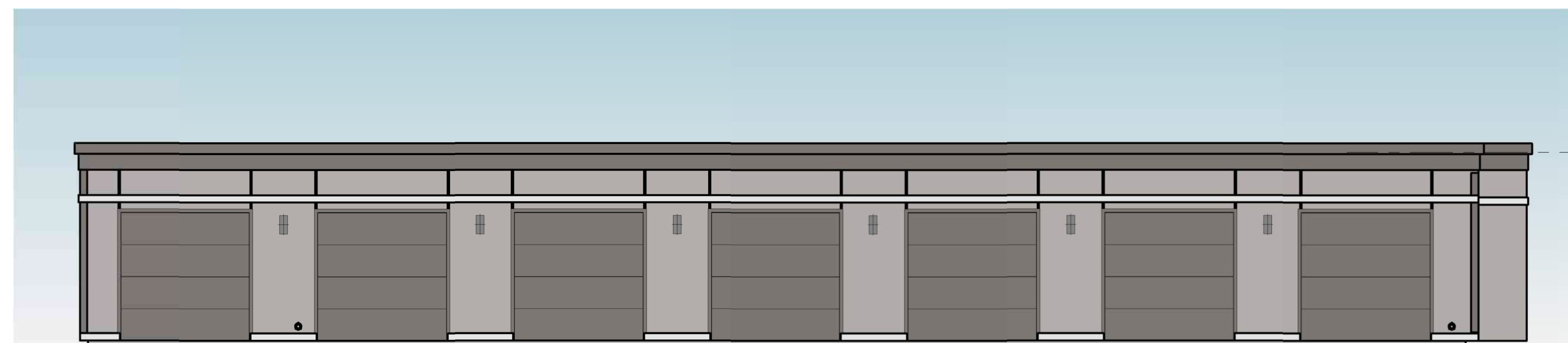
7 BAY GARAGE FRONT ELEVATION 3/16" = 1'-0"
